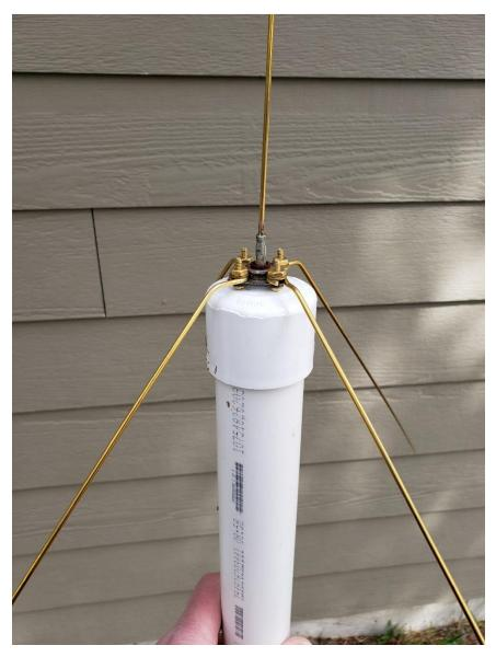
This is a simple and inexpensive antenna for use on the two meter band. The antenna is relatively easy to build and effective. It also has the merit of being inexpensive.
