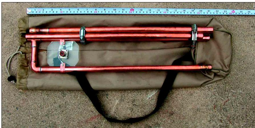
**Figure 7—The completed folding J-pole, ready for packing.**
