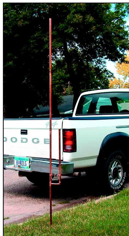
need to tie a large enough knot in one end of the bungee cord so it won't pull through an eyebolt. Run the bungee cord through an eyebolt, through the other pieces of copper pipe, and place the eyebolt cap in the copper pipe, tapping the copper cap into place. Make sure that the couplings are facing down, so that when it rains the antenna doesn't fill with water.
